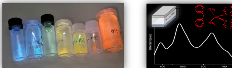
Figure. Design of copper complexes for rainbow emission and white LECs application
